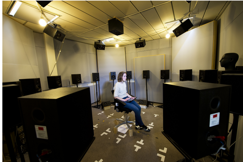
Figure 2.1: Photograph of the ‘Spacelab’ at DTU. A spherical array of 29 loudspeakers allows for the auralization of acoustical scenes in virtual rooms. Photo: Joachim Rode.
