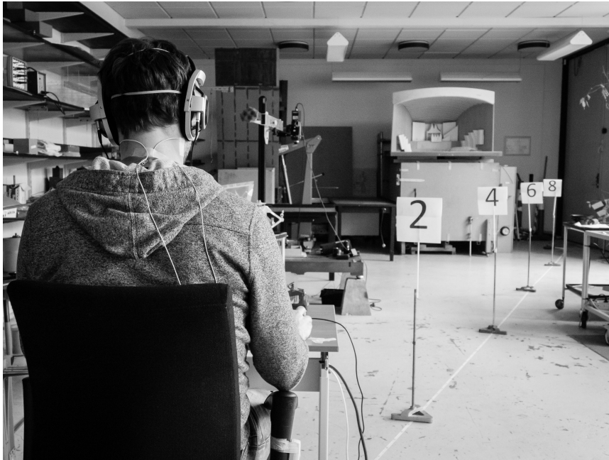
Figure 4.1: Photograph of the listening test setup in a workshop room with dimensions 12.7 x 6.8 x 3.1 m and a reverberation time T_{30} of about 0.7 s. Stimuli were presented via Sennheiser HD800 headphones, and visual distance markers were provided at 2, 4, 6, and 8 m.
