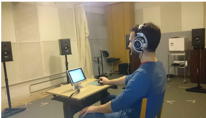
Figure 5.2: Photograph of the experimental setup with a listener at the listening position inside the IEC listening room. The four loudspeakers were positioned at 0, 25, 60, and 90° at a distance of 2.5 m. The listeners controlled the experiment via a graphical user interface on a small screen using a wireless mouse.
