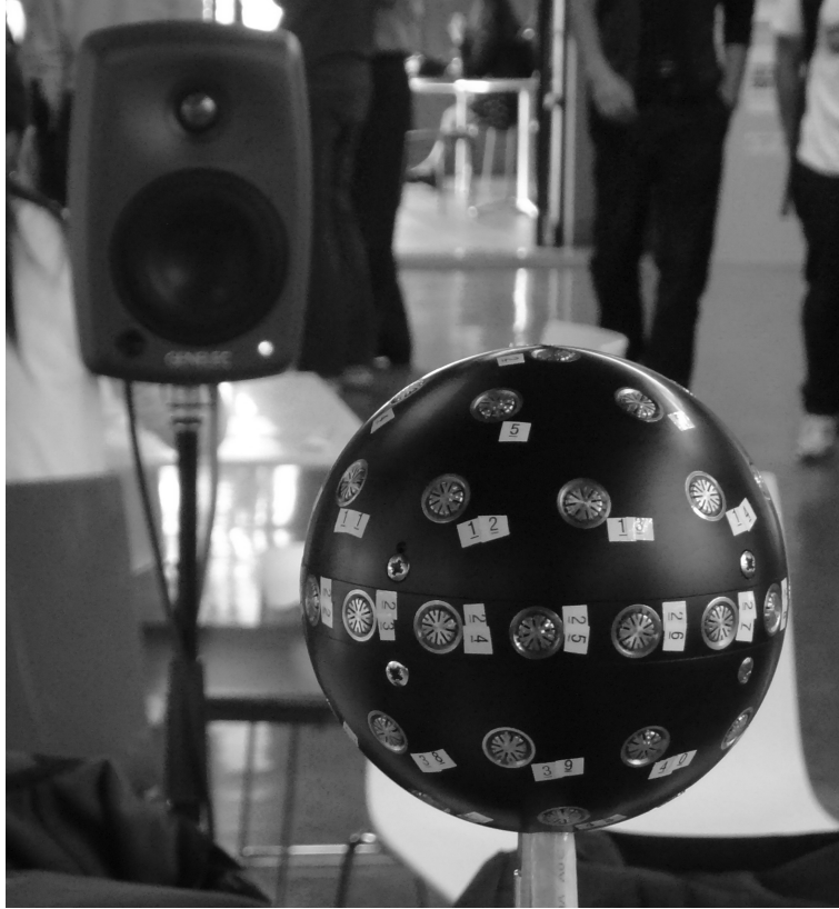
Figure 3.1: The realized 52-channel mixed-order ambisonics microphone array.
