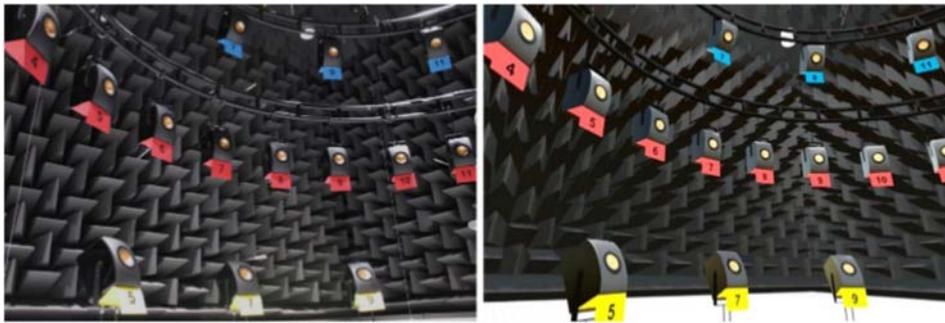
Figure 4.1: Photography (left) and screenshot (right) of the acoustic reproduction system in the real (RE) and in the virtual environment (RE and VE). The loudspeakers are numbered in azimuth and color coded in elevation.
